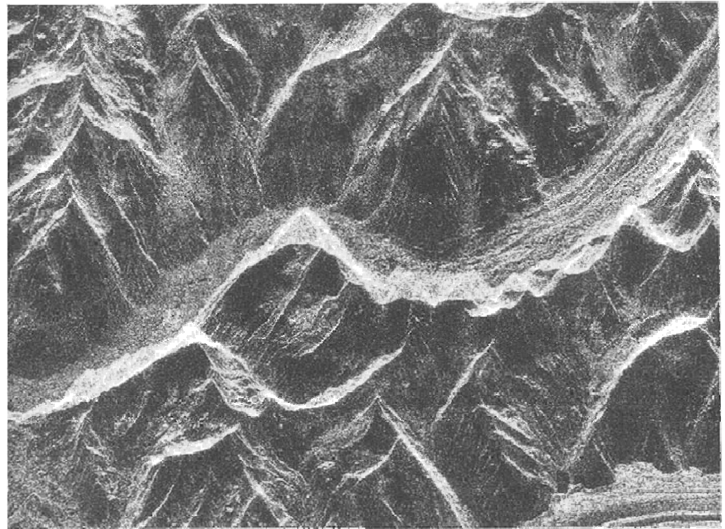
Figure 5-4. Example of radar image layover. Seasat image of the Alaska Range showing the top of a mountain imaged onto the glacier at its foot (center). Shadows are also present on many of the backslopes of these steep mountains. Illumination is from the top [from Ford et al., 1989].
